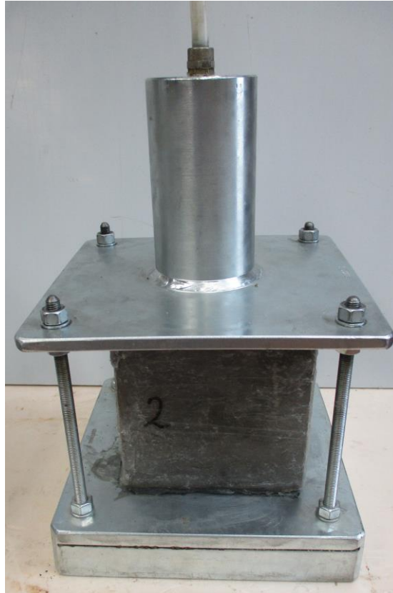
Figure 3. Experimental apparatus for measuring water permeability under pressure.
